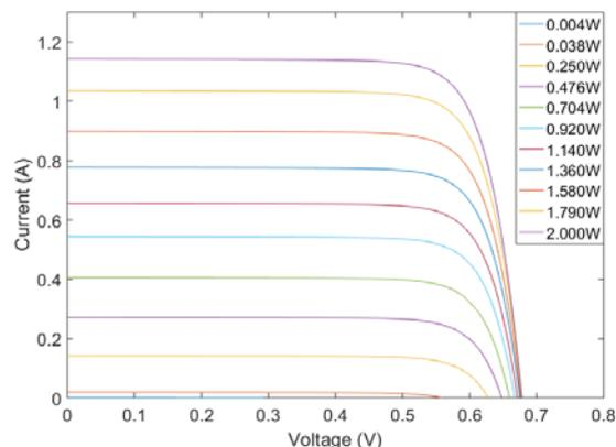
Figure 3. Current-Voltage measurement of the LPC while illuminated by an 808 nm wavelength laser beam.
