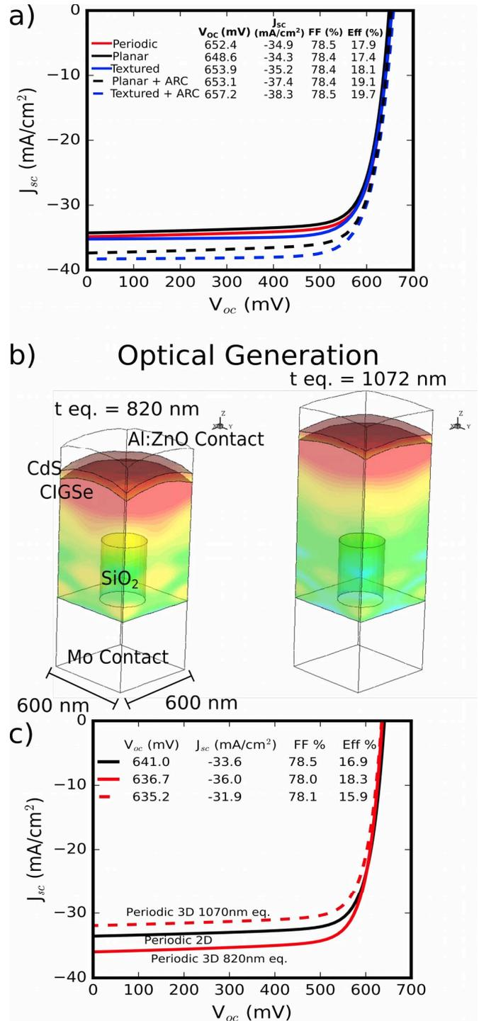
Fig 3: a) The simulated JV curves for the three architectures with the addition of a  $190\text{nm}$  dielectric separation layer with point contacts. Also, an ARC is applied to the planar and textured devices with the dielectric layer. b) Optical generation in one unit cell of a conformally deposited CIGSe device onto a square lattice of dielectric cylinders with two different thicknesses of absorber. c) JV curves comparing the 2D model to the 3D model of the devices in b).
