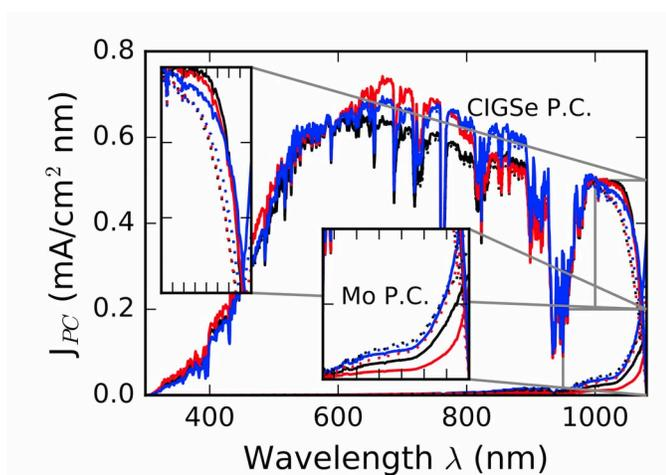
Fig 2: The absorbed photocurrent under AM1.5-G illumination of different device architectures, random (blue), periodic (red), and planar (black) are shown without (dashed curves) and with (solid curves) dielectric separation layers.
