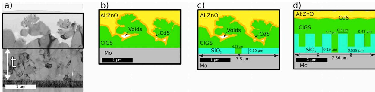
Fig 1: Simulated Cross-Sections: a) A representative focused ion beam (FIB) cross section of randomly textured CIGSe absorber films is used to define the photovoltaic model, shown in b). In c), a SiO<sub>2</sub> layer serves to increase reflection and define electrical contacts.
