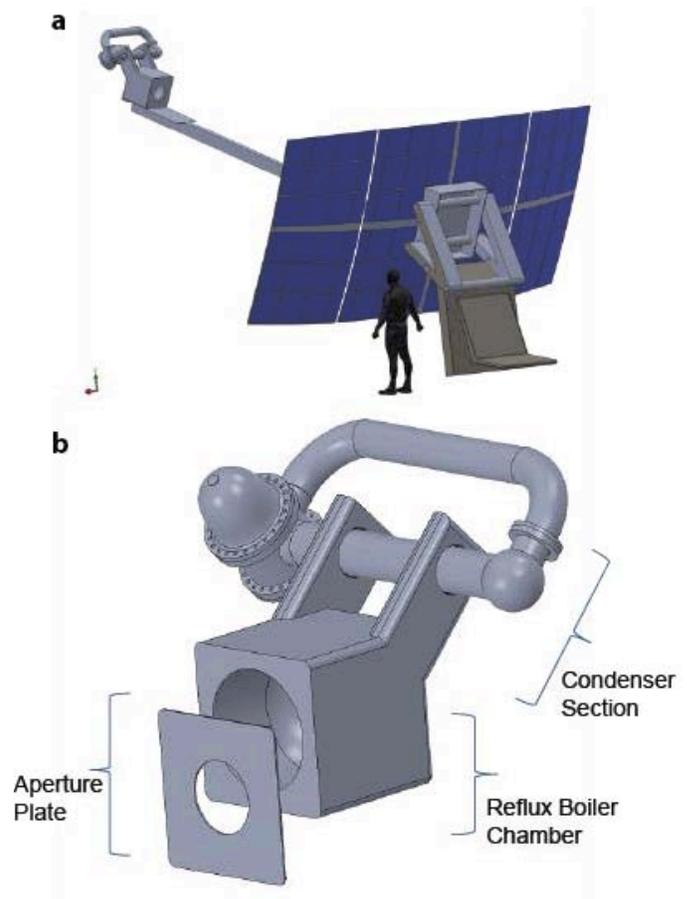
Fig. 1. (a) Overall system including parabolic dish concentrator and (b) detailed FSSS.
