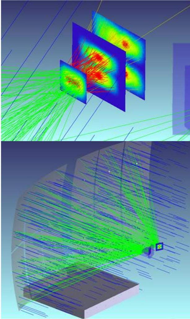
Fig. 2. Ray optics modelling of the incoming sunlight into the parabolic dish concentrator and focused into the concentrator solar cells (CPV) mounted on the copper plate.
