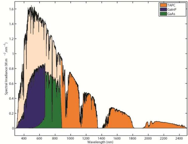
Fig. 3. Full usage of the solar spectrum with photovoltaics conversion from the solar cell and thermal energy conversion from the waste heat of both the solar cell and the mid- to far-infrared part of the solar spectrum that can't be converted by photovoltaics.
