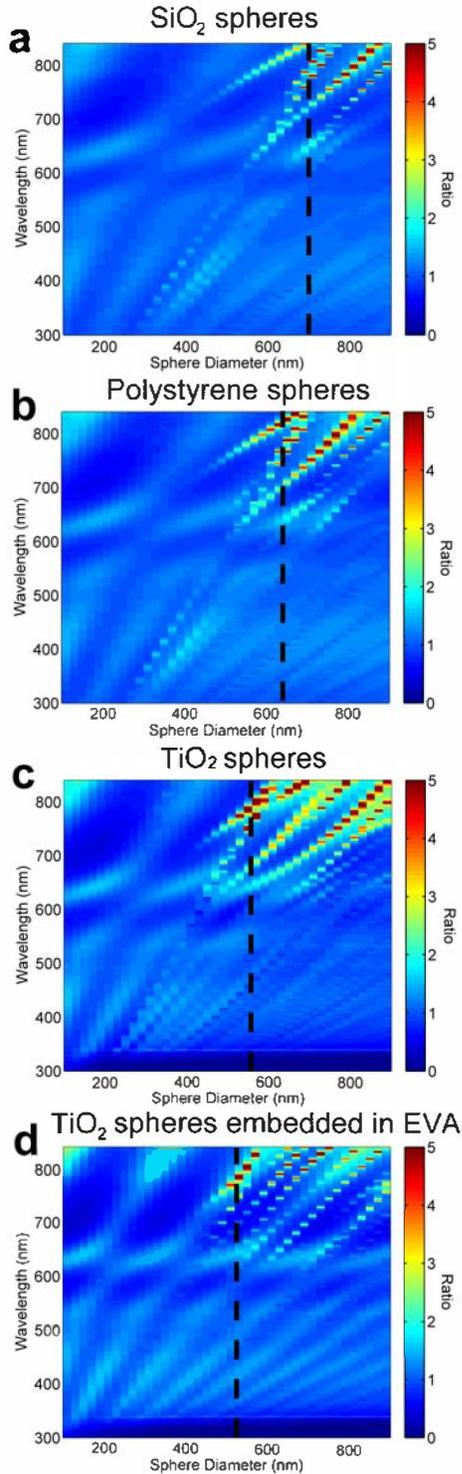
Fig. 2. Ratio between the spectral current density of an a-Si silicon solar cell with HCP spheres over the spectral current density of a solar cell without spheres for (a) SiO<sub>2</sub>, (b) polystyrene, (c) TiO<sub>2</sub>, and (d) TiO<sub>2</sub> embedded in EVA. The dashed black line shows for each case the sphere diameter which gives the highest current density when illuminated with the solar spectrum.
