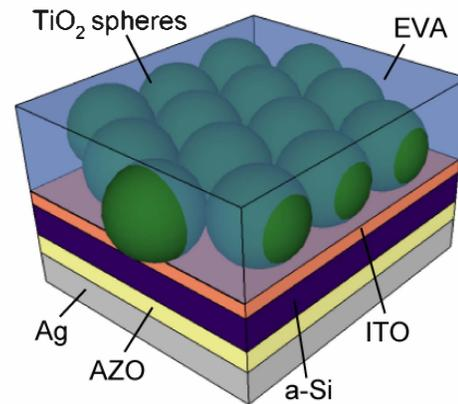
Fig. 1. Schematic of the solar cell with  $\text{TiO}_2$  spheres embedded in EVA.
