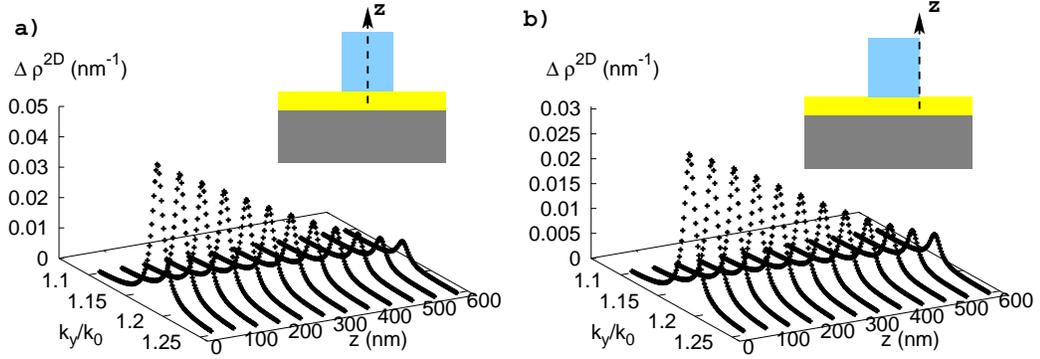
Fig. 2. LDOS calculated at the waveguide center (a) and edge (b) in function of both normalized propagation constant  $k_y/k_0$  and height  $z$  in the dielectric strip. DLSPPW is a  $w = 400 \text{ nm} \times h = 600 \text{ nm}$  polymer strip ( $n_d = 1.5$ ) on a  $40 \text{ nm}$  thick gold film. The wavelength is  $\lambda = 1.55 \mu\text{m}$ .
