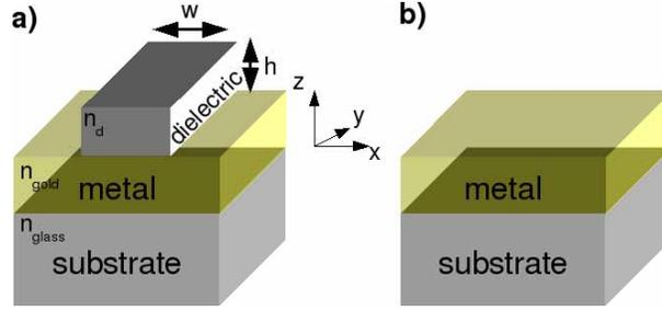
Fig. 1. a) DLSPW configuration. A  $w \times h$  dielectric strip (optical index  $n_d = \epsilon_d^{1/2}$ ) is deposited on a gold film, supported by a substrate. b) Corresponding so-called reference geometry consisting of the same system without the dielectric strip.
