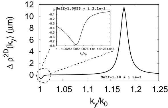
Fig. 3. 2D-DOS variation in function of wvector component  $k_y$  along the DSLPPW axis. The inset shows a zoom near the Au/air SPP mode effective index.
