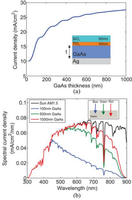
Fig. 2. (a) Current density of a flat GaAs solar cell with back reflector and double antireflection coating as a function of the GaAs thickness. (b) Calculated spectral current density for different GaAs layer thicknesses. The spectral range is weighted by the solar spectrum and compared with the AM1.5 solar spectrum.
