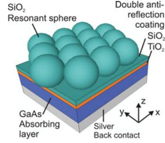
Fig. 3. Schematic of a GaAs solar cell with hexagonally close-packed SiO<sub>2</sub> nanospheres on top of it.
